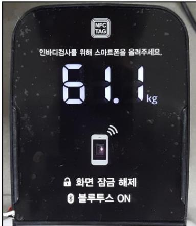
3. When you come down from the foot plate, the weight will be 0.0kg and will automatically turn off after 5 seconds.
